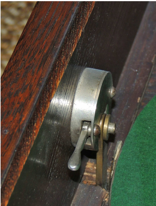
Fig 4: Re-set lever on inside front of case
