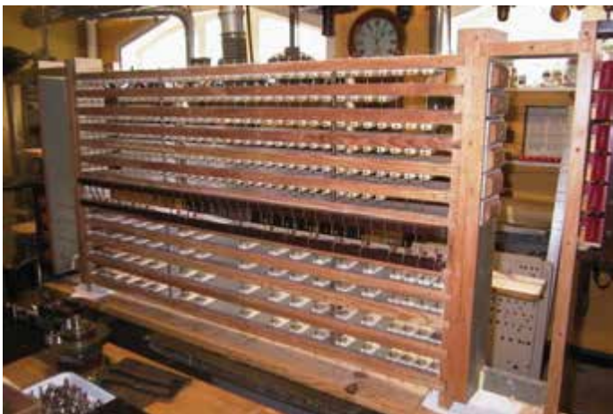
Fig 23 Replacing pull wires, pallet valves & toe board gaskets
