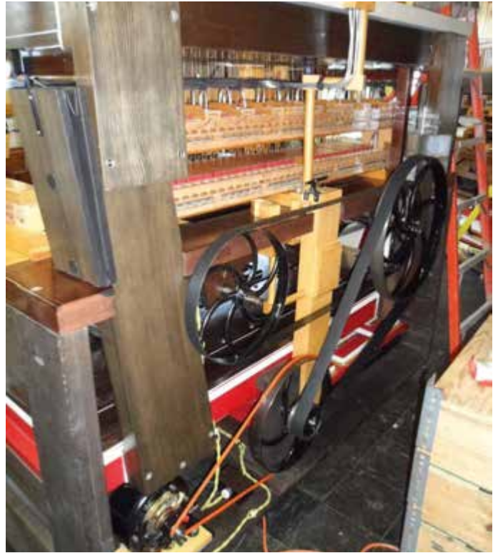
Fig 41 Motor & belting installed
