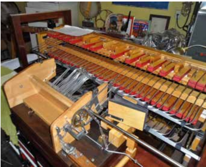
Fig 38 Tin tubing connecting tracker bar to pneumatic stack
