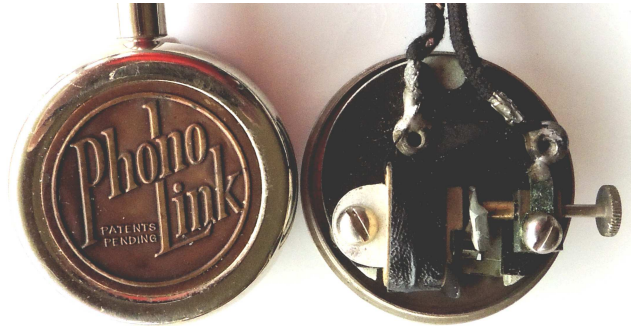
Fig 10: The inside of the Phono-link (right) showing the horseshoe (C-shape) permanent magnet with the insulated wire coil slightly to the left at the bottom. The "volume" knob (at the right) simply forces the armature/needle holder against a strong flat spring until it is central in the air gap. This does, no doubt, change the volume, at the expense of any lateral compliance the thing might have had, and at the expense of extreme wear on any record played using the device.
