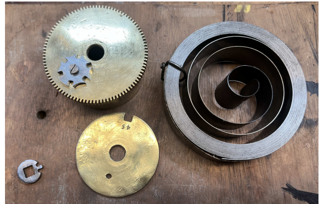
Fig 4: Showing the new mainspring before shortening. the comb also needed tuning.
