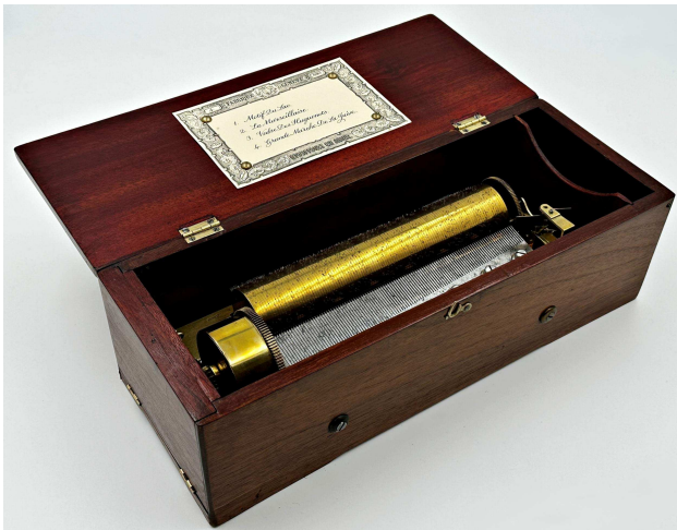
Fig. 3A. Another 4-air key-wind single comb movement with the name Valogne stamped upside-down on the bedplate, Fig. 3B. Serial number unknown but estimated as 1840s.
