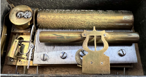
Fig 4: Showing the zither and the mandoline pining on the right end of the cylinder
