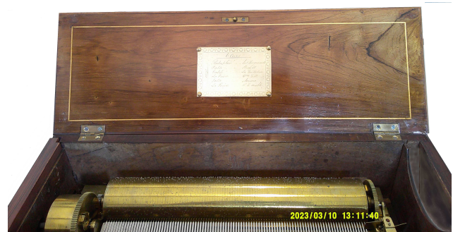
Fig 3.1B: Movement and tune sheet of Henriot 6-air box.
