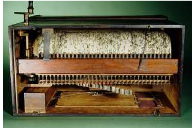
Fig. 5B. A view of the barrel, key frame and arrangement for Fig. 5A.
