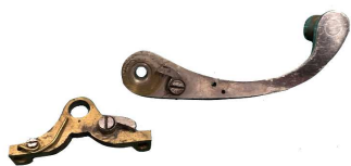
Fig 5: Ratchet click springs of wire!
