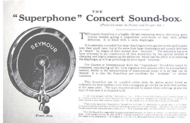
Picture 3: Superphone Concert soundbox, which was fitted with a mica diaphragm.
