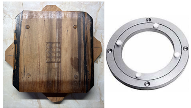
Figs. 13 & 13A: Home-made turntable and bearing
