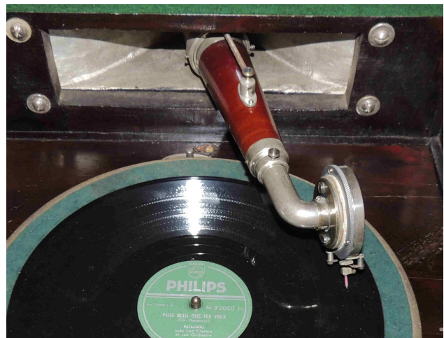
Picture 1: Seymour tone arm with 'counterbalance spring'.
