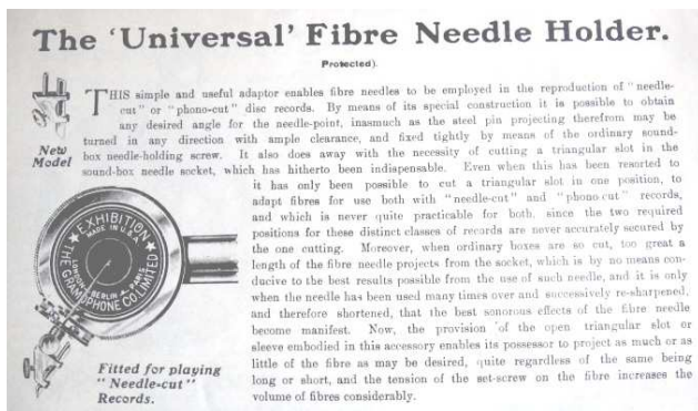
Picture 8: A useful accessory - a special fibre needle holder for triangular bamboo needles - that could be attached to any soundbox - shown on a HMV 'Exhibition' box.
