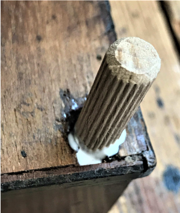
Picture 8: A new dowel ready for the leg to be fitted
