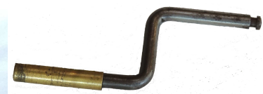
(Above): The original re-wind crank, the end doubling as a reed puller.
