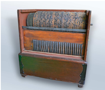
Fig 4: The pallets and barrel of the barrel harmonium
