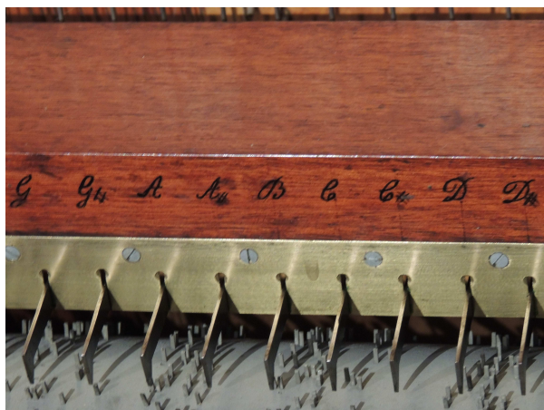
Fig 2: The keyframe with tuning scale marked
