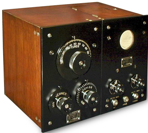
Fig 1: The two-stage Westinghouse model RC radio used in the Lyradion cabinet.
