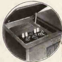
Sectional view of top of cabinet showing installation of Radiola III-A.
