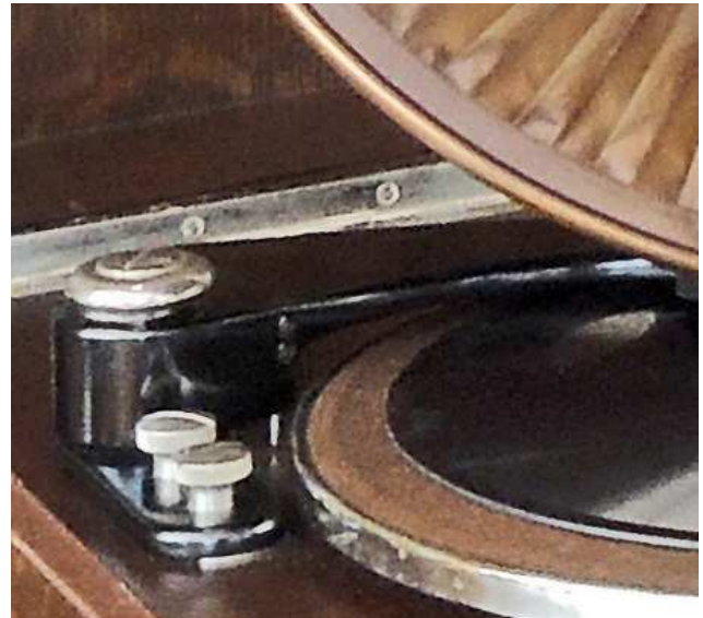
Fig 12: Showing the knurled mounting bolts.
