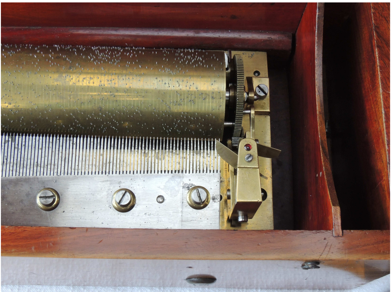
Fig 2: Showing the top eleven teeth on a separate steel plate
