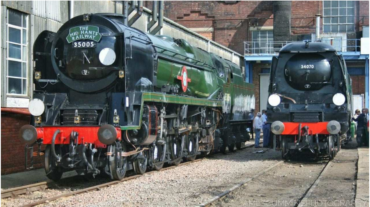
Bulleid Pacific locomotives for the Southern Railway. The example on the left is a re-built one with Walschaerts valve gear.
