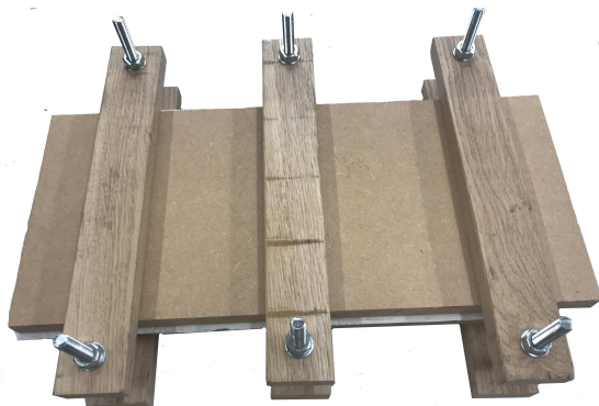
Fig 6: The home made veneer clamp
