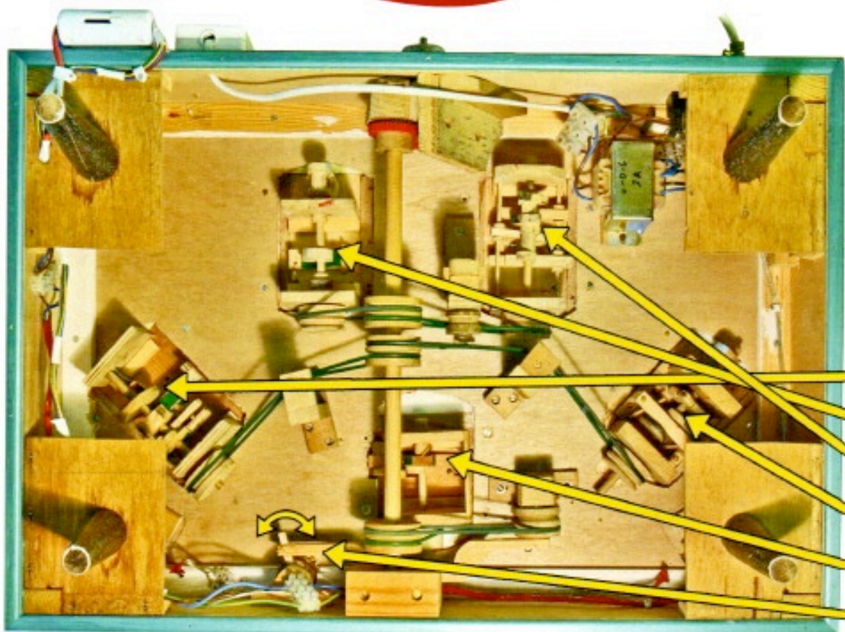
The belt-driven hand-cranked mechanism.
