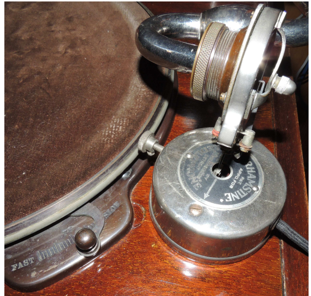
Fig 7: The Needlephone in use on a gramophone.
