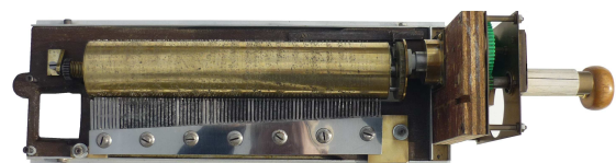
Fig 6: The repaired comb in position
