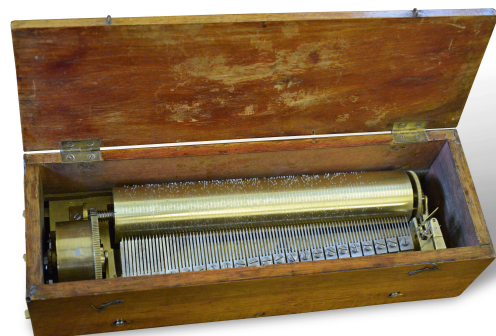
Fig 7: Sectional comb of Ducommun-Girod 13172
