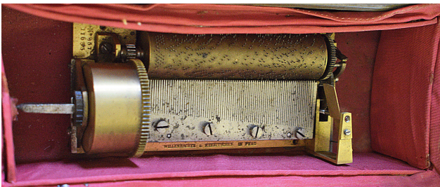
Fig 12: The movement by Willenbacher & Rzebitschek in Prag
