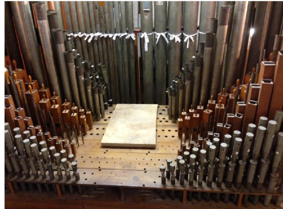
Fig 4. Main windchest and some of the ranks
