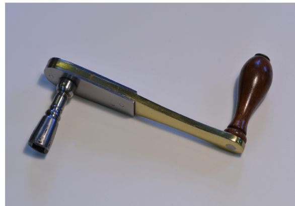
Fig 3. The ratchet-wind 'key'.
