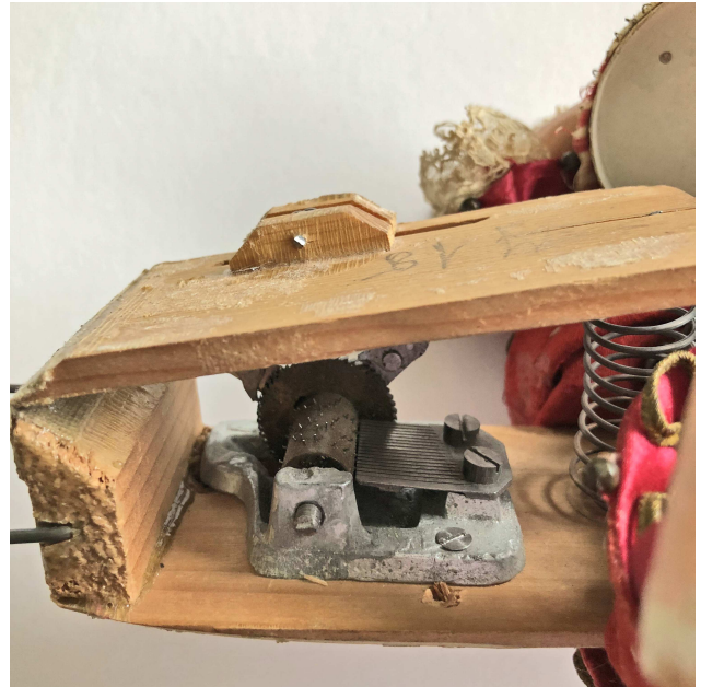
Picture 4: A single tune pinned on the barrel
