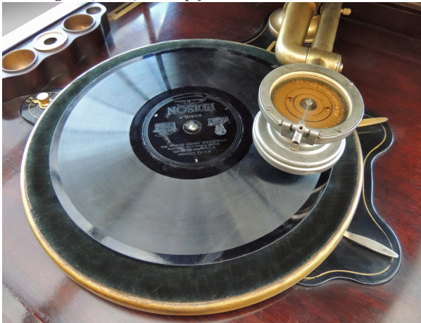
Fig 1c (below): Set up for Edison Diamond discs
