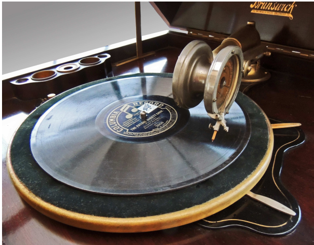
Fig 1a: Brunswick Ultona soundbox set up for needle-cut records. The tone arm is telescopic, to set the tracking.
