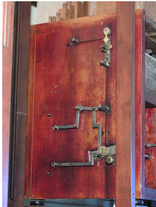
Picture 4: The feeder crank arrangements
