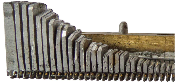
Fig 6: Bass lead tuning marks
