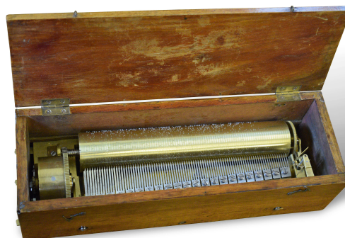
Fig 7: Sectional comb of Ducommun-Girod 13172
