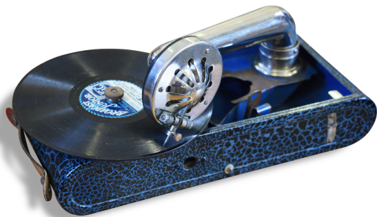
Fig 4: 'Excelda' in playing mode. The soundbox is based on the HMV 5A.
