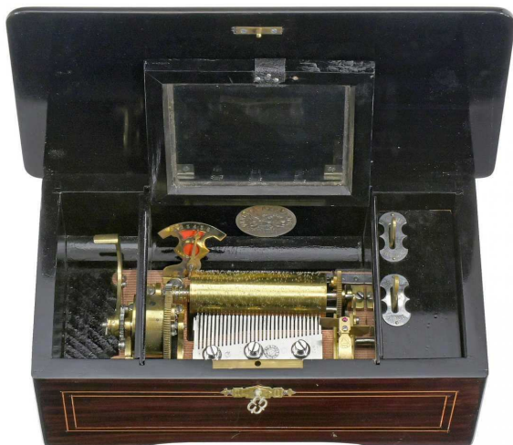
Picture 1: Small Ullmann box with 31 teeth
