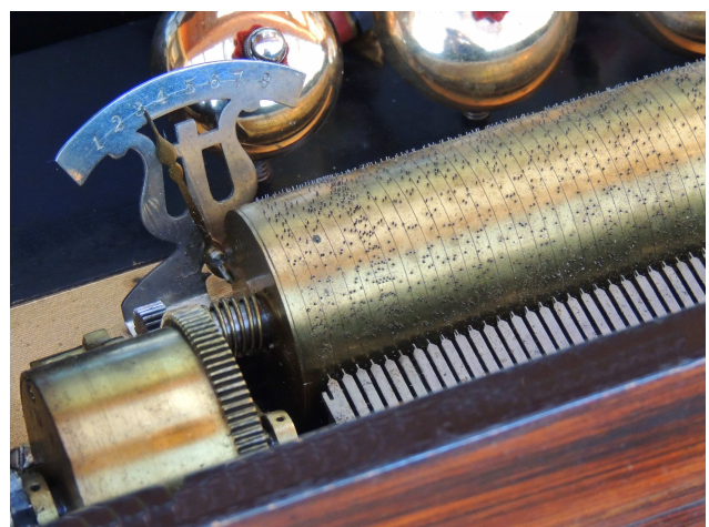
Picture 9: The cylinder pins which operate the conductor's arm and baton can be seen in front of tooth no. 6
