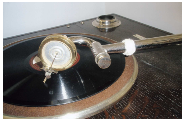
The Turk's Head knot - the soundbox rests on it when folded back.
