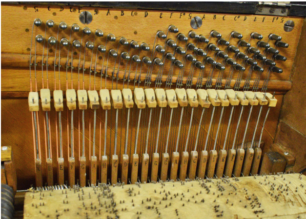
Fig 9. 'Proper' felt piano hammers
