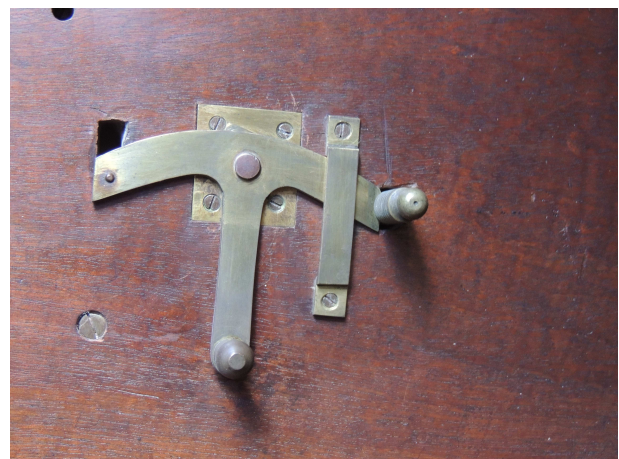
Picture 5. The tune change device.
